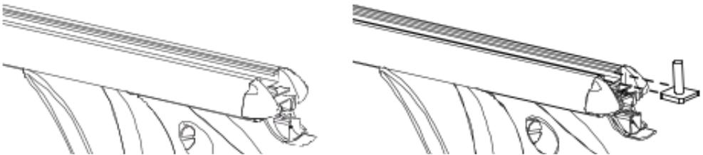
End cap can be opened to remove the rubber strip & insert T-Bolts for ease of adding accessories. You will need to cut the rubber strip to reinsert around the T-Bolts, and maintain the weatherproofing of the roof bars.
